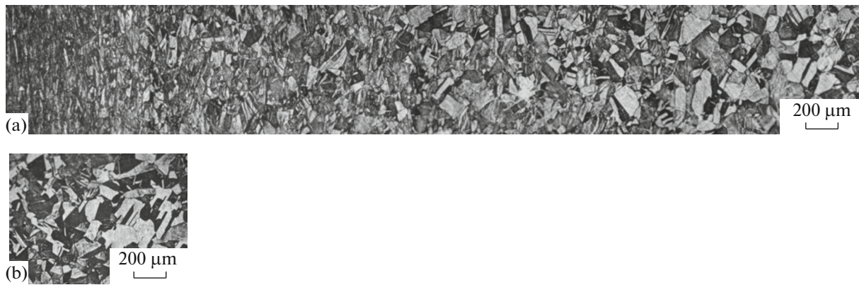
Fig. 3. Microstructure in the billet cross section after four TE passes: (a) 5-mm-long panoramic image taken along the diameter of the hexagon in the direction from the edge to the center of the cross section (from left to right) and (b) center of the cross section.
