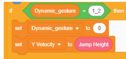
(b) replacing the control with a variable that stores the number of a previously recognized dynamic gesture
